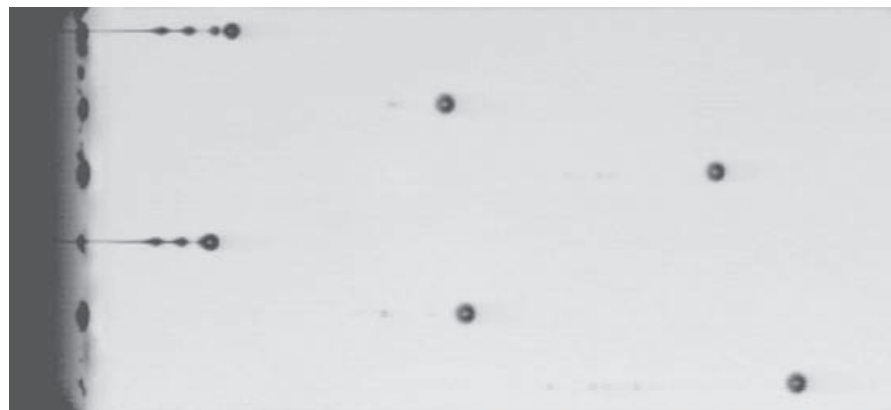
Figure 2: Grayscale ink drops: small droplets join together to create a variable-sized drop
